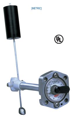
(%" — 24 x %"), for attachment to a gauge adapter with 2.5" [63,5] diameter bolt circle (see Rochester Adapter Machining Standard MS-502). Model 6280 and 6283 Senior gauges used on above ground ASME storage tanks are equipped with direct-reading 5001S00001 percentage dials.
