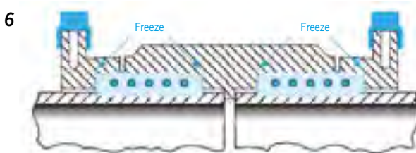
Melt solidifies at the start of the cold zones, thereby sealing the melt zone. Further input of energy causes increase in melt pressure.
